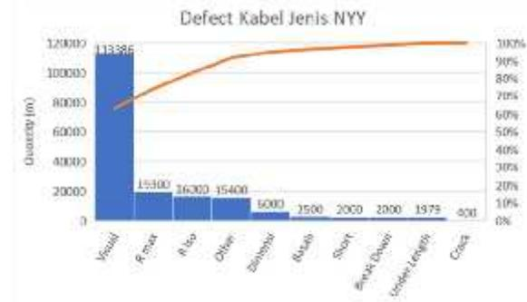
**Gambar 1.** Diagram Pareto Perbandingan Defect Kabel NYY
