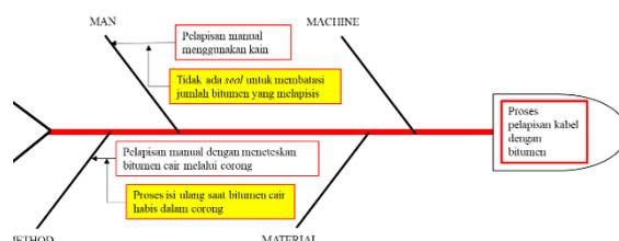
Gambar 10. Fishbone diagram analisis proses pelapisan bitumen
