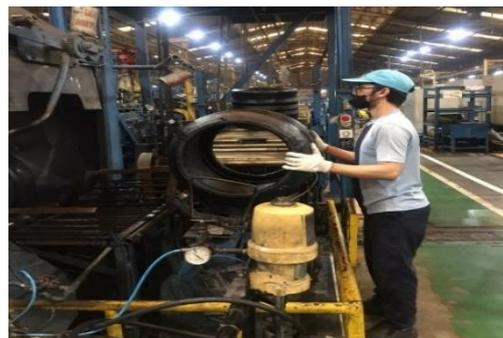
Gambar I. Kondisi Awal Proses *Transferring Green Tire* Pada Mesin VTT-4
