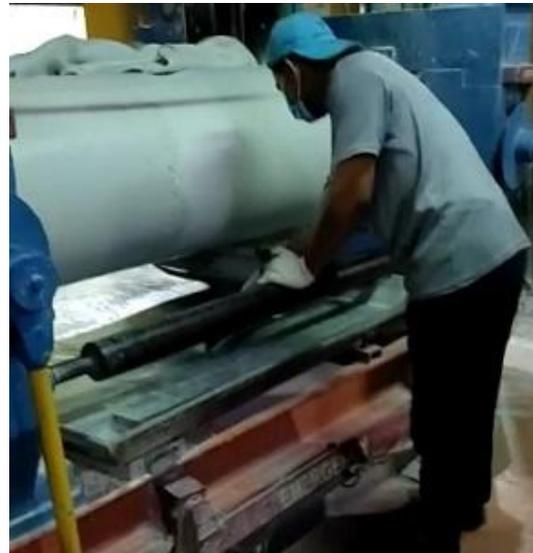
**Gambar 1.** Setting Pisau Cutter Open Mill Manual
