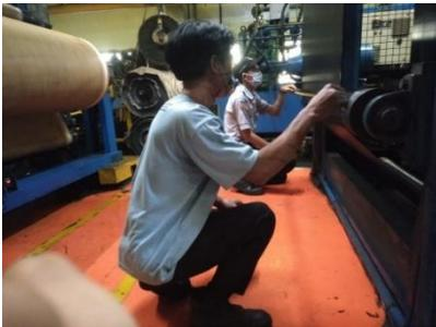
**Gambar 1.** Postur Badan Operator *Topping Calender* Saat Melakukan Pengukuran Lebar *Treatment*
